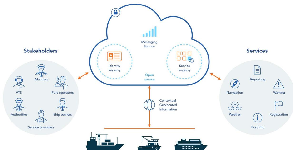
*Figure 1 - Overall Concept of the Maritime Connectivity Platform*
